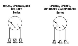
**Contact Ratings:** SPDT center off; 2 A, 30 VDC, 1 A, 125 VAC pilot duty.
