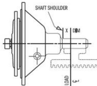
**RC214 & RC314P - ALLOWABLE SIDE LOAD KG (LBS)**
