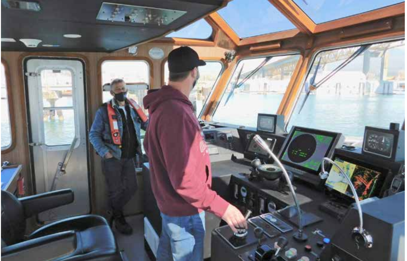
Capt. Brendan Maxwell takes the controls with Z-drive training master Capt. Ryan Scott watching over. Scott, who retired from Seaspan in November 2019, likens driving a Z-drive tug to operating a skiff with a tiller-steered outboard. "If you pull the tiller one way, the boat goes other way." The TEMPEST's wheelhouse doors (and other doors and hatches) are from Earl's Marine Closures, with windows from AdvanTec and wipers from Northwest Marine Distributors.
