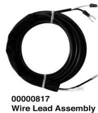
**Wire Lead Assembly** 00000817 is a 14 ft. (4.27 m) extension with mating plug connections for the 00000818 and 00003488 thermocouples. The wire is PVC covered, non-shielded, 18 AWG (1.0 mm<sup>2</sup>), with heat shrinkable sleeve provided for insulating terminals after installation. Extension up to 100 ft. (30.48 m) can be made with 18 AWG (1.0 mm<sup>2</sup>) or larger copper wire at the gage head.
